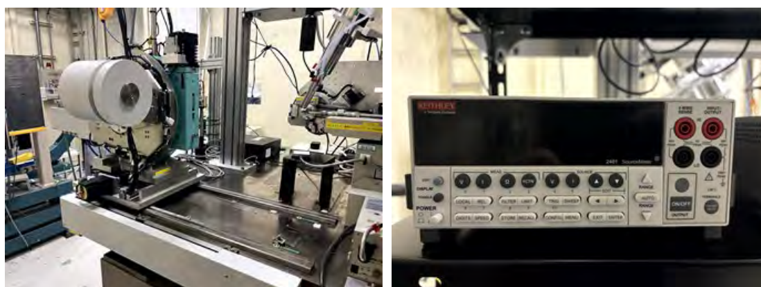
Fig. 1. Diffractometer without the imaging plate detector for the single-crystal X-ray diffraction measurement (left) and a source meter (right).
